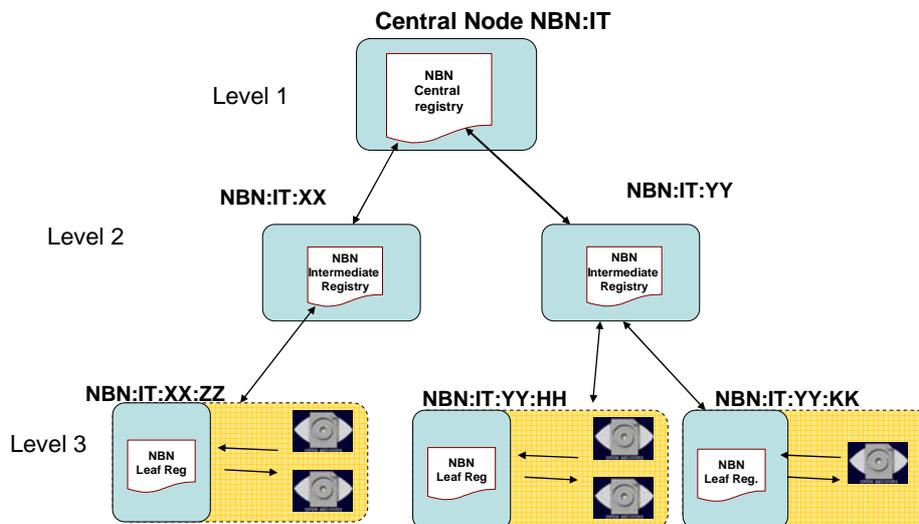
**Figure 1: The multi-level distributed architecture**
